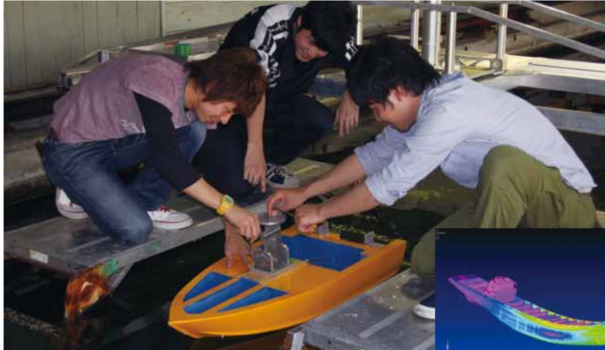
●Preparation of high-speed planing boat performance test.
