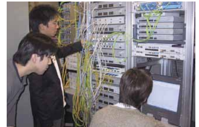
●Packet Transmission Experiment in IP-over-WDM Network.
