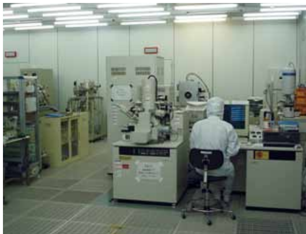
●Class 100 clean room.
